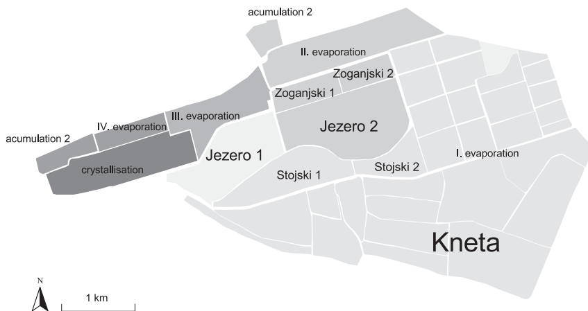
Fig. 5: Nomenclature of basins (salt-pans) of different evaporation grades and local names for different parts or salt-pans in the Solana Ulcinj.
