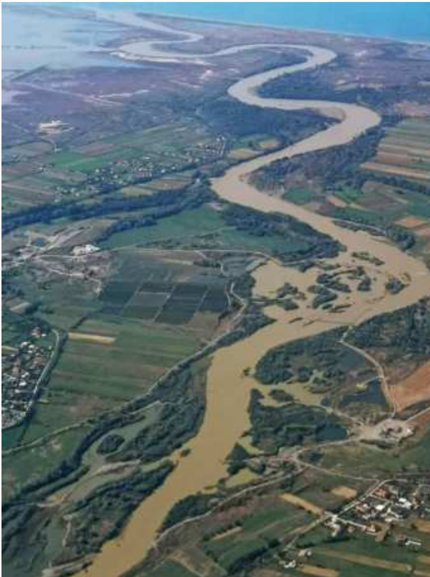
Figure 2: The sediment transport from the mountains to the coastal plains in all grain fractions, particularly coarse material, is essential. The Matí River -due to the blockage of larger grain fractions (i.e. gravel) by several larger dams only transports fine suspended material. This becomes particularly evident by the muddy colour of the river.
