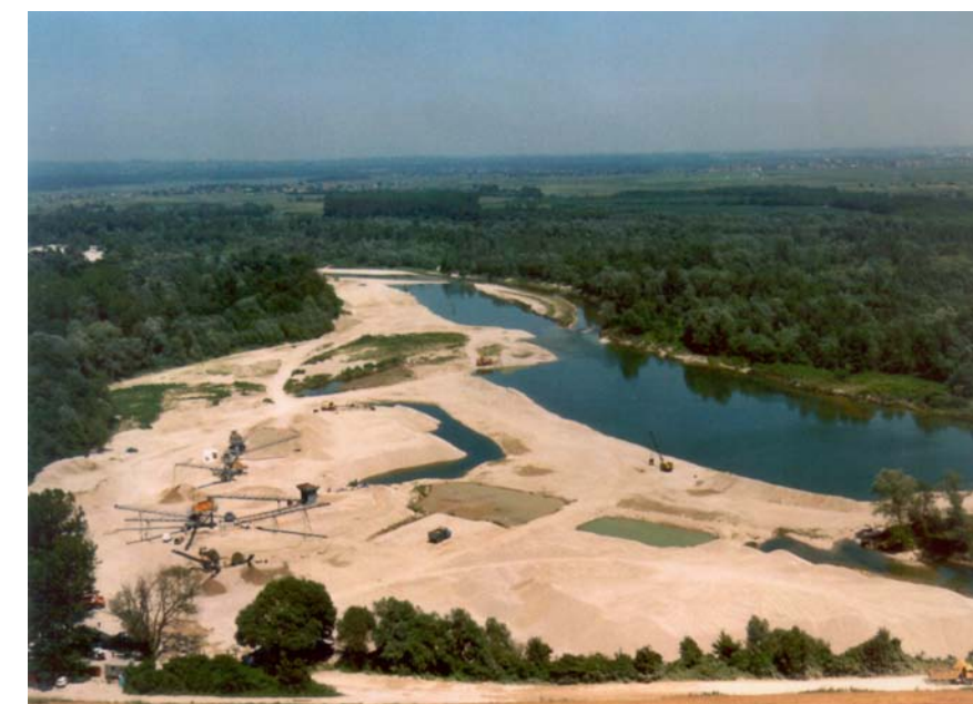
Fig. 38: Intensive gravel excavation and destruction of the former Drava river bed near Varaždin (Credit: ZEUS)
