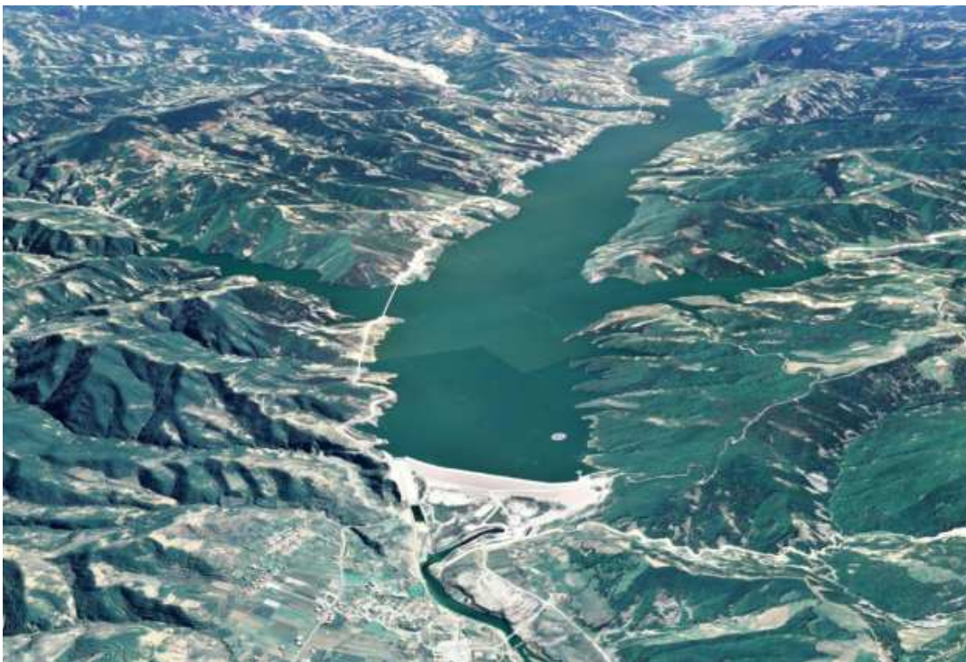
Figure 4: Large dams, such as this one on the Devoll River in Albania, trap a significant amount of coarse sediments. This leads to downstream consequences, including substantial bed incision and a reduced flow of sediments reaching the deltas—in this instance, the Semani Delta (Google Earth 2023).
