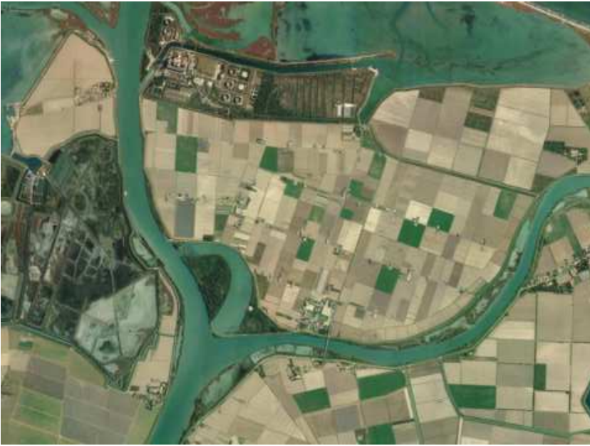
Figure 8: Examples of river regulations in the delta area: fixation of riverbanks, meander cut-offs, construction of canals with sluices and outlets and the disconnection of floodplains by dykes (agricultural or even industrial usage), the case example from Po Delta (Google Earth 2023).
