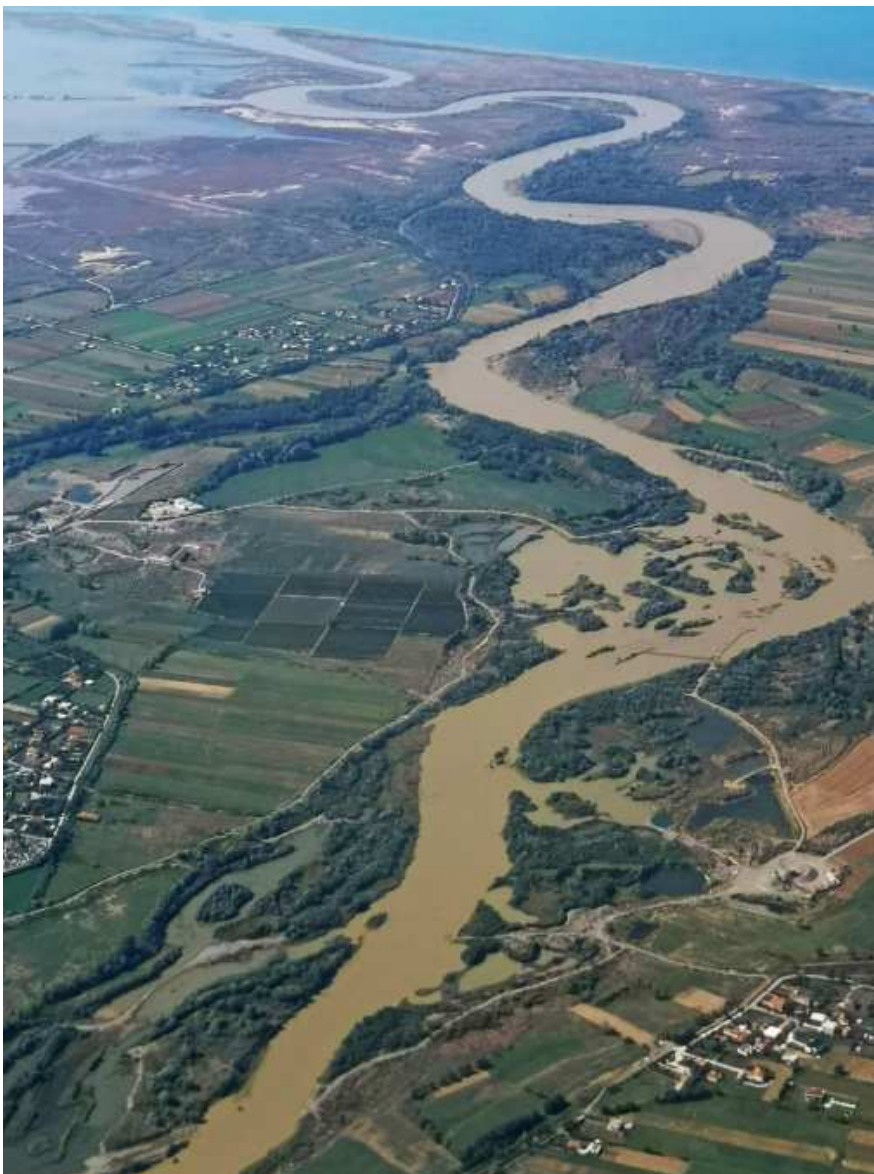
Figure 2: The sediment transport from the mountains to the coastal plains in all grain fractions, particularly coarse material, is essential. The Mati River -due to the blockage of larger grain fractions (i.e. gravel) by several larger dams only transports fine suspended material. This becomes particularly evident by the muddy colour of the river.
